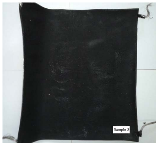
Figure 1. Image of 307 mm \times 300 mm silicone-CNT mat with connected electrodes. [Color figure can be viewed in the online issue, which is available at wileyonlinelibrary.com .]
